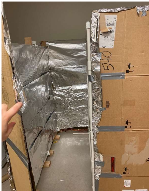
Figure 4.3 Aluminum foil reflective front walls from cardboard.
