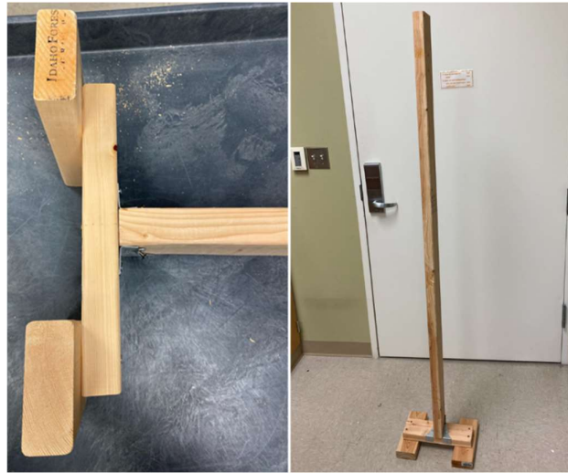
Figure 2.2 Attaching the upright section of the stand.
